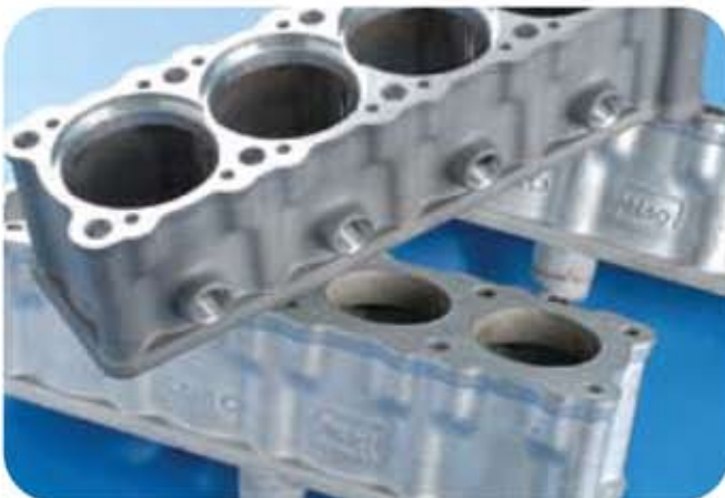
T-Mag magnesium motorcycle engine block castings; upper casting fettled and partially machined; lower castings after sand core shakeout.
