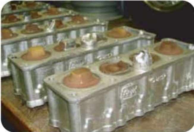
As-cast magnesium motorcycle engine blocks, showing small sprue and sand cores.
